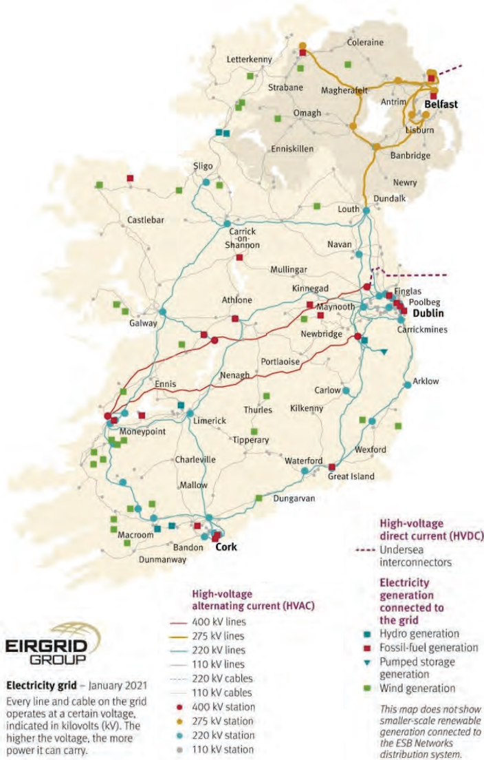
FIGURE 2: EIRGRID ELECTRICITY GRID NETWORK
